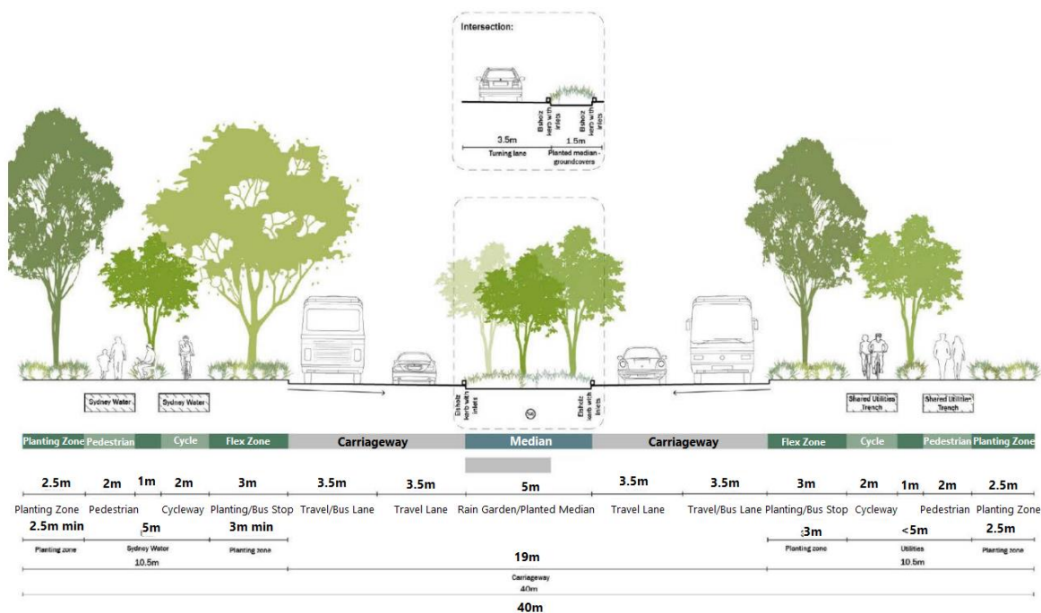
Figure 13 - Sub-Arterial Road Typical Section
