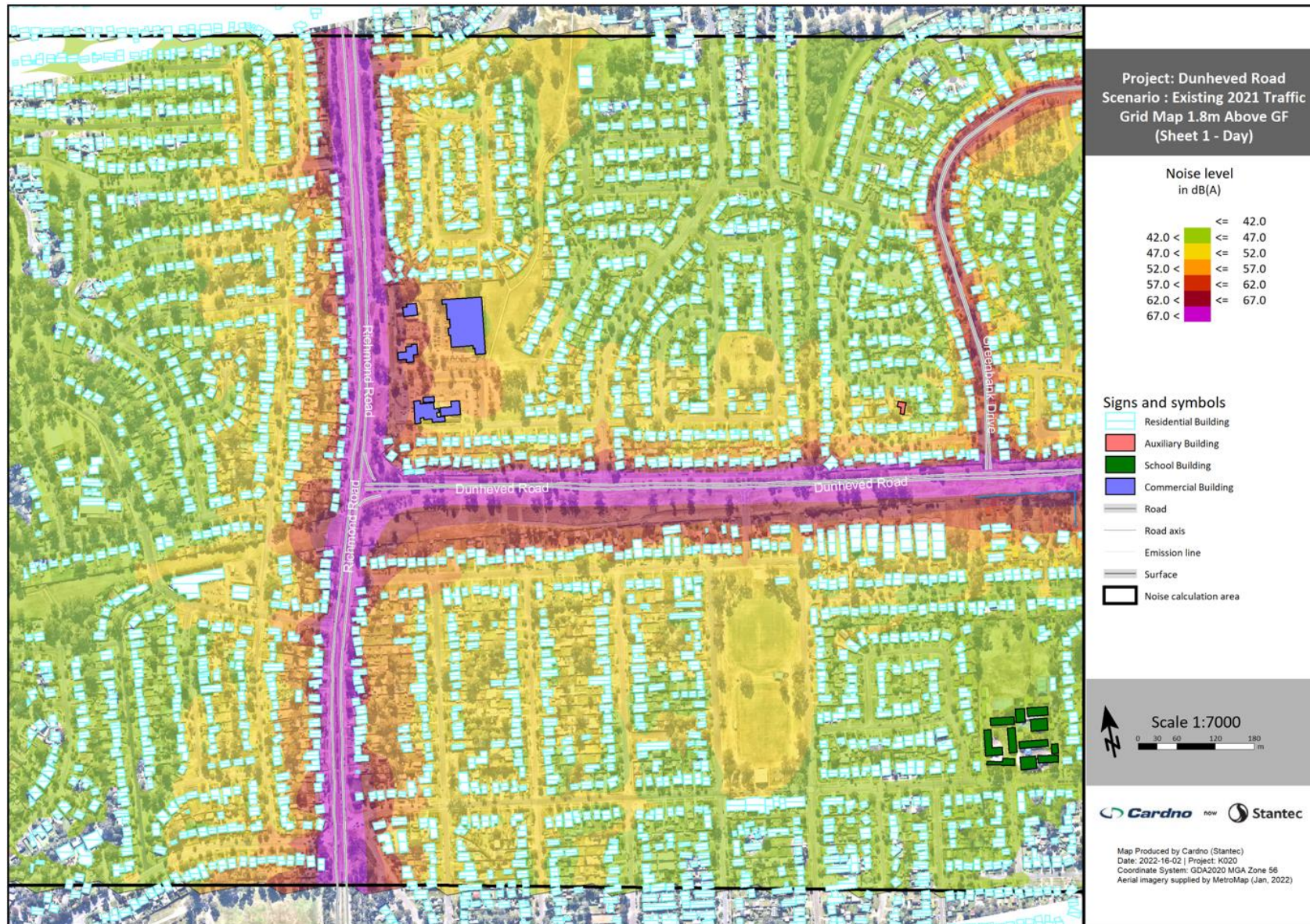
Figure 7-1 Existing Traffic Noise Levels – Day – Western Extent
