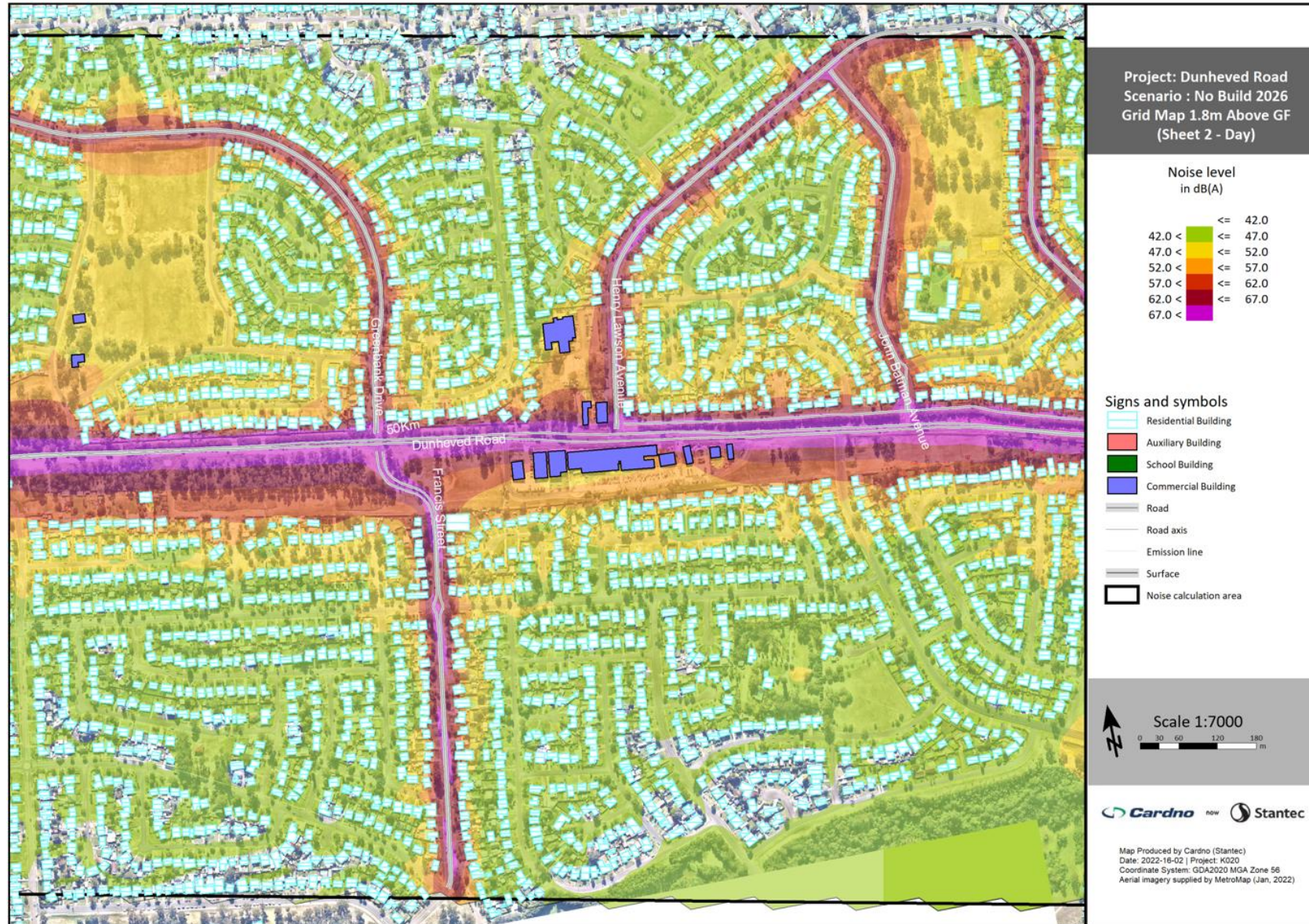
Figure 7-5 Year 2026 – No Build - Traffic Noise Levels – Day – Central Extent
