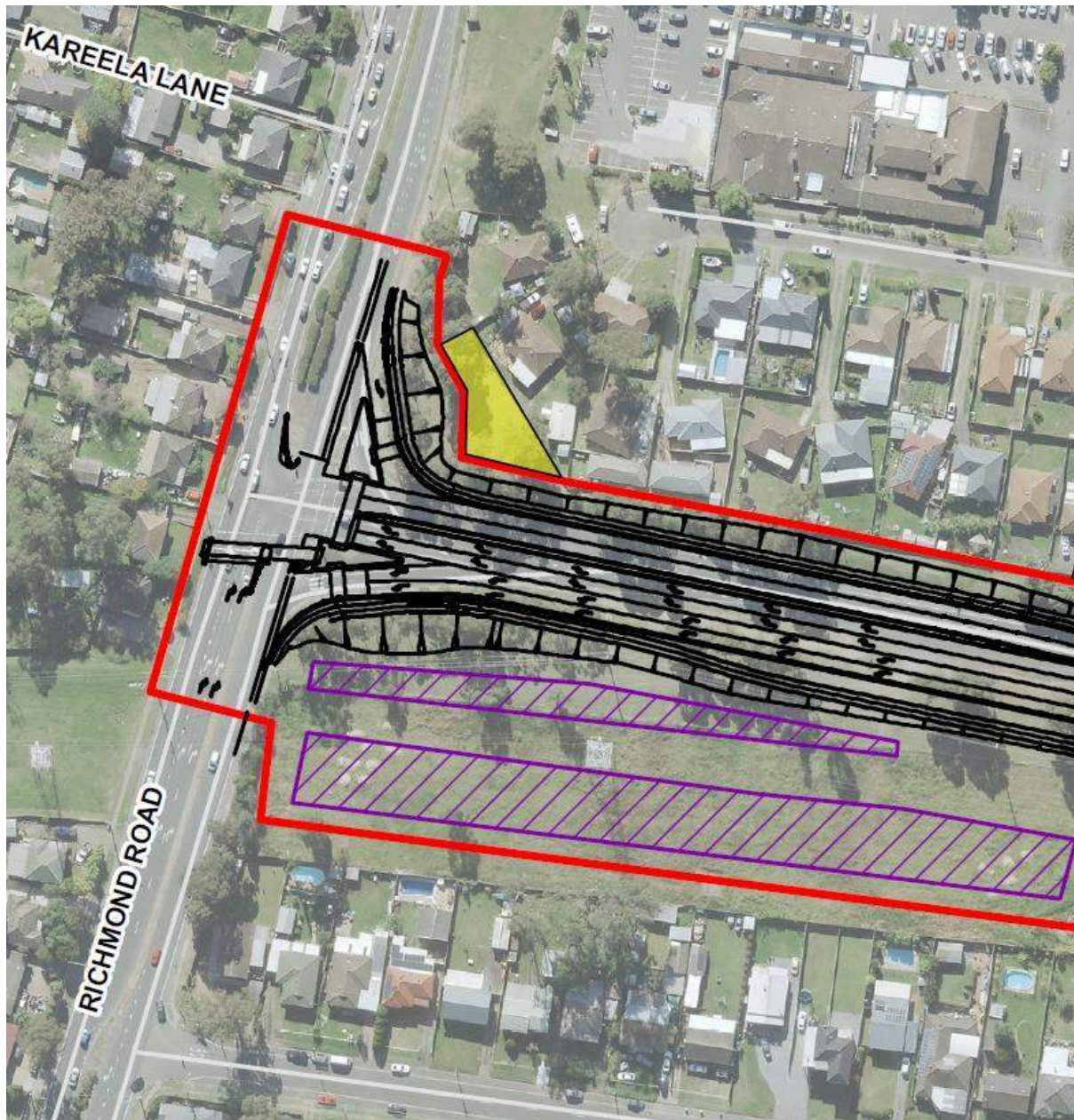
Figure 3-1 Location of additional noise barrier
