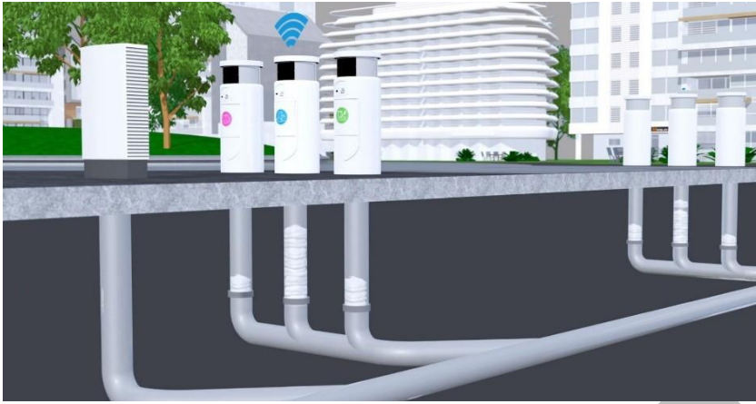
Figure 56: Free standing inlets and supporting underground networks for the transportation of waste items
